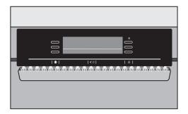
As soon as the oven is started, the SpeedLight lights up yellow. The rising temperature is shown by the change in the colour of the light from yellow via orange to red.
